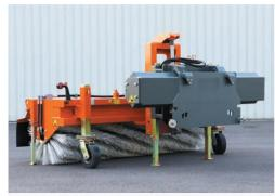
bema 3 Robust with hydraulic lateral movement
