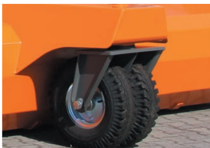
Sturdy twin wheels with reinforced rim (Super-elastic solid rubber wheels Ø 446 x 122 mm)
