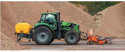
bema 35 Dual PowerMaster equipped with collection container Dual including scraper unit, high-pressure water unit, water tank in the rear and certified camera system (see page 58/59)
