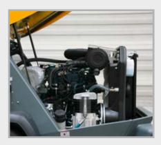
The powerful diesel engine with 28 kW and diesel particulate filter complies with the requirements of the exhaust emissions standard "Stage V". The air required for spray applications is provided by the compressor.
