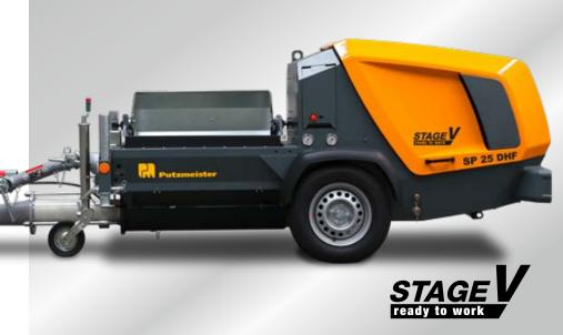
The powerful SP 25 DHF auger pump is suitable for conveniently and reliably placing large volumes of self-levelling floor screed. Thanks to the strong three-cylinder diesel engine with 37 kW and "Stage V" emissions, the pump can be operated without issues in the whole of the EU and Switzerland now and in future. The increased efficiency focuses on higher throughputs, longer delivery ranges and higher delivery pressures.
