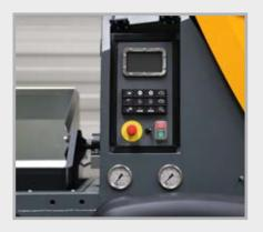
The central control panel with intuitive keypad increases operating safety. A clearly structured display behind scratch-resistant protective glass supplies the machine operator with all relevant information.
