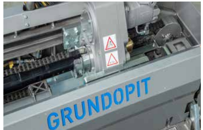
ROTARY DRIVE WITH QUICK ROD CONNECTOR
