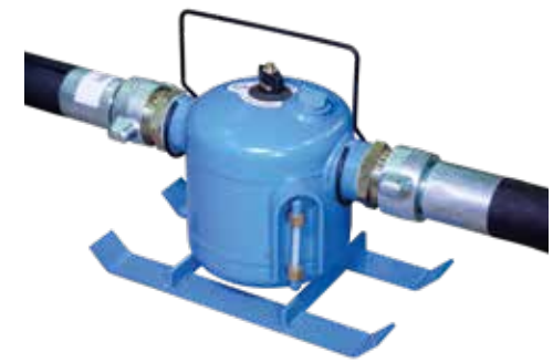
THE 7-L OIL LUBRICATOR is installed between the compressor and the machine to enable lubrication of the internal piston.
