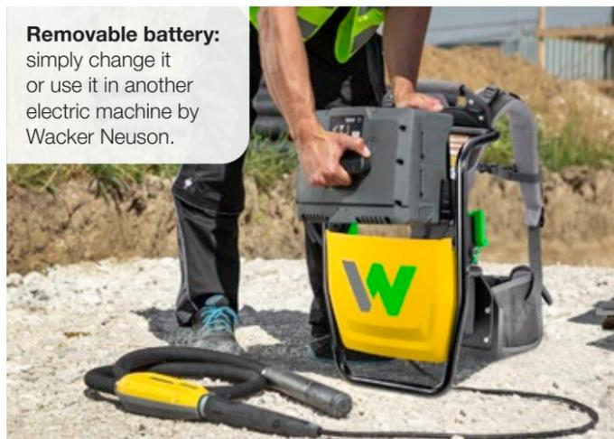
**More safety on the construction site:** no more long power cables landing in wet concrete or becoming a tripping hazard.
