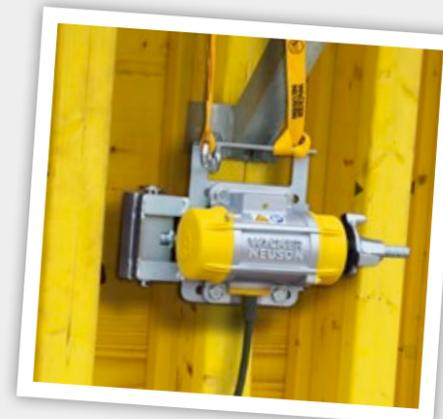
**Loosening and separating** bulk material in a silo.
